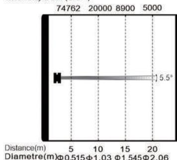
Max. Beam Mode Intensity LUX (46°)
